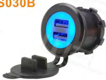
Input: DC12-24V USB output: 5V 4.2A Material: ABS/PA+hardware Product Size: 37*29*53mm USB output selection: 3.1A/4.2A Light color: RD/BU Shell color: BK/WH
